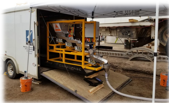
The Micro Doser MD3+ delivers ACE XP Polymer Fiber™ continuously to either the Drum or Pug Mill
